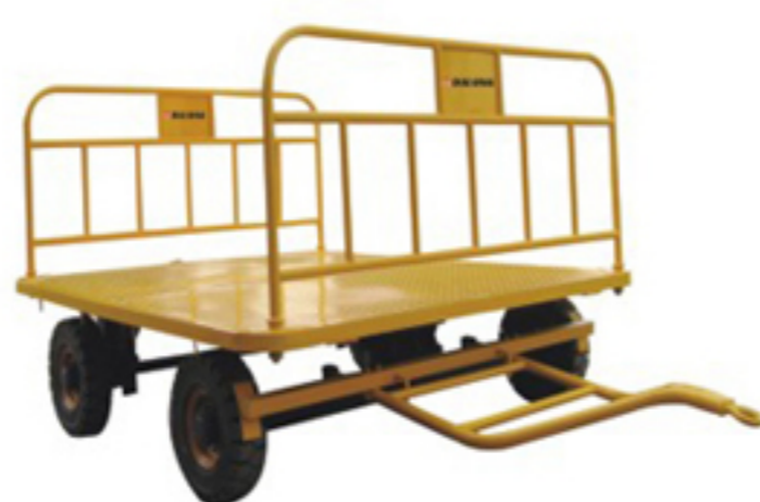
QD-G平板拖车(牵引车用) Capacity:2000 Kg Dimension:2400 x 1200 mm
