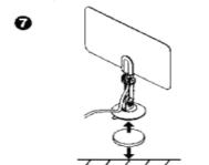
4.Use the optional multi-stick pad to fixed the antenna base on a unfinished surface. (figure 7)
