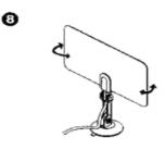
5.Horizontally adjust the antenna position left or right for a better reception. (figure 8)
