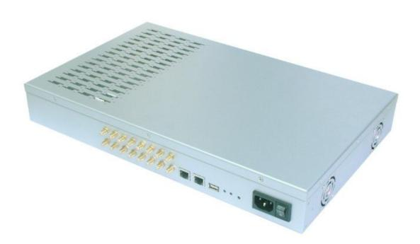
GSM VoIP gateway ETS16x8G is newly designed IP to GSM gateway supporting maximum 16 ports 128SIMs of GSM Voice interface, it can effectively realize the smooth transition between PLMN(GSM) and VoIP network. Compact cost effective design and system architecture of GSM Gateway ETS-16x8G provides customer satisfaction in high quality , performance and system reliance.
