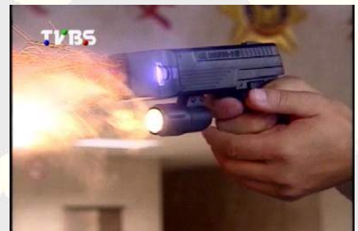
Cartridges of probes/ pepper powder/ pepper bullet / rubber bullet/ paint/ S.O.S signal bullet fired out and Xenon Light on for illumination, giddyding & target acquisition.
