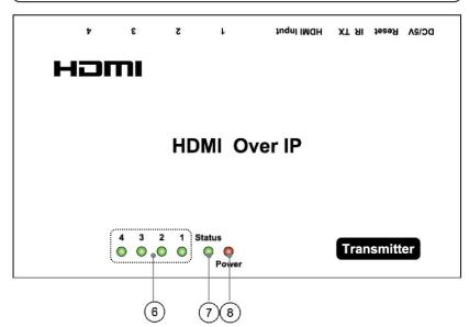
Link ports HDMI input IR-TX port
