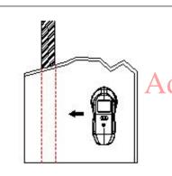
Without releasing on/off button, slide scanner in reverse direction to locate the other edge of stud. Mark this second spot. Middle of stud is centered between the two marks.
