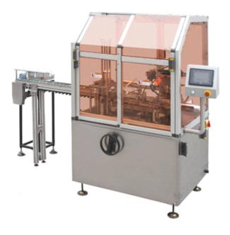
Automatic cartoning machine is used for putting medicine bottles/boards/unguents into the folded cartons and then closing the ends of the cartons. Some models of the cartoning machines have additional function of seal labeling and shrink wrapping.Infeed entrance usually can be divided into three: one for manuals, one for medicine bottles/boards/unguents and one for cartons.
