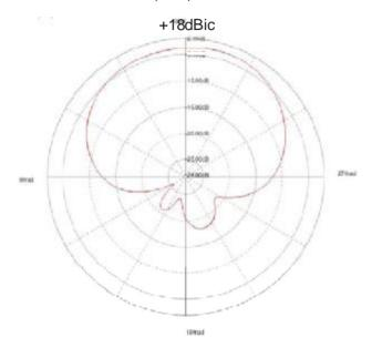
The GeoHelix-M, with optimised LNA gain and low-noise figure, provides a typical gain and Noise Figure of 18dBic and 1.6dB, respectively.
