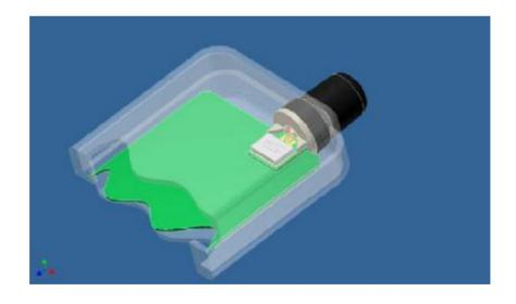
GeoHelix-M antennas may be mounted externally or embedded within a device. When mounting externally, the groove in the radome should be used as a mechanical support. For further information on integrating the GeoHelix-M, please refer to the integration guideline.
