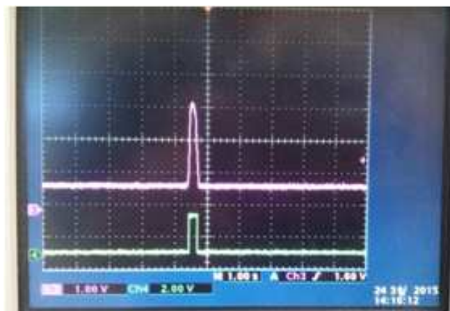
Fig. 2 Typical \alpha -decay signal (up) from detection circuit and converted trigger signal (down) (1s/div, 1V/div)
