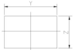
Snap-in Panel Cutout X=Panel Thickness
