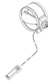
Battery operated electro-balance damper with remote control, cable through drywall with termination fixture, no distance limite
