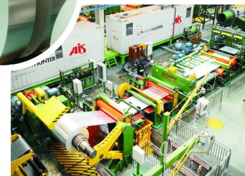
法塔拉矫清洗线 FATA Tension Leveling and Cleaning Line
