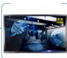
FHD touch screen A+ grade 1.07B colour original panel,10-point-touch,1920x1080 FHD,AWB TECH Suit for universal application scenarios
