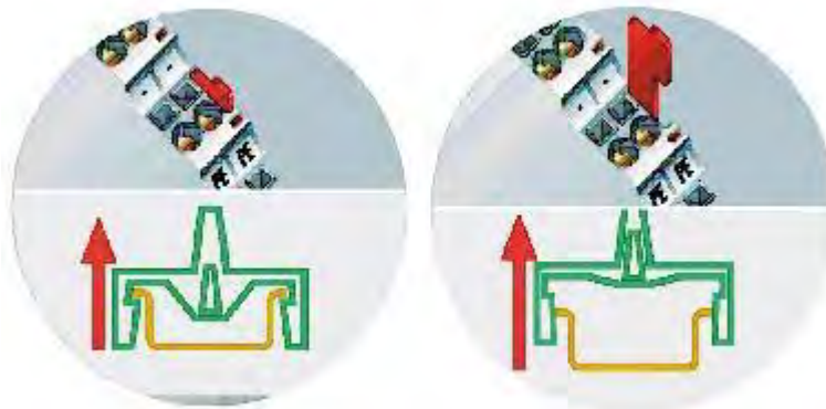
Figure 2.3 GCAN-PLC-400 self-locking mechanism
