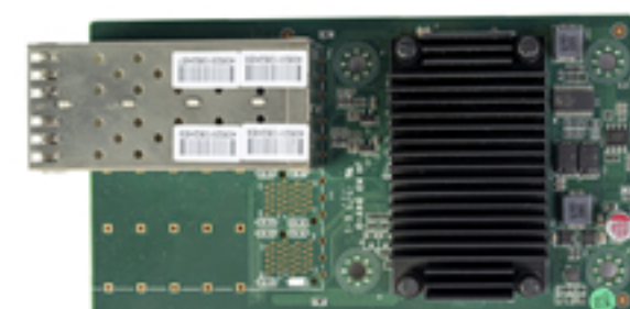
4*I350 SFP Gigabit Ethernet
