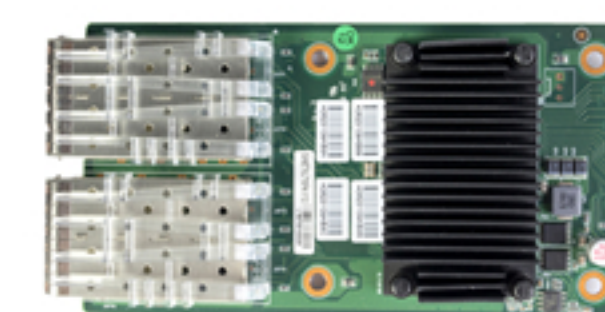
4*X710 SFP+ 10 Gigabit Ethernet
