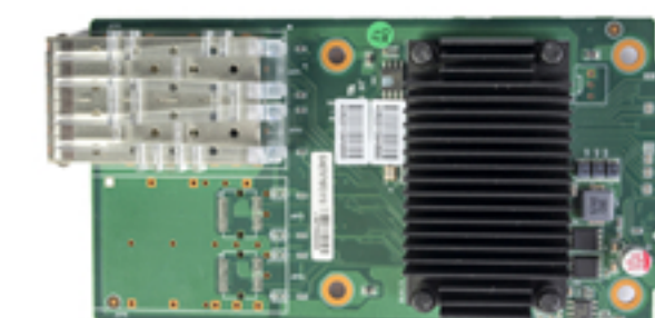
2*X710 SFP+10 Gigabit Ethernet
