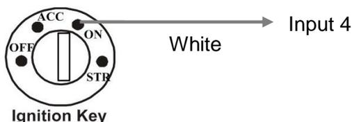
Input 4 is connected to ACC ON position to detect the engine ON/OFF status;
