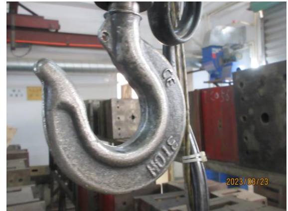
NC 7.17 No safety latch for the hoist
