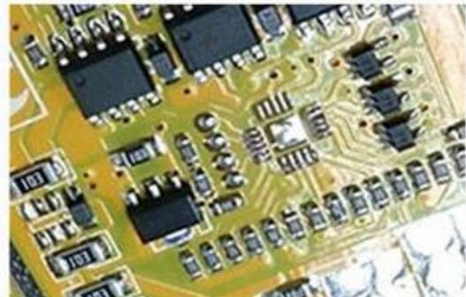
Mix Mounting Of Resistance-Capacitance IC
