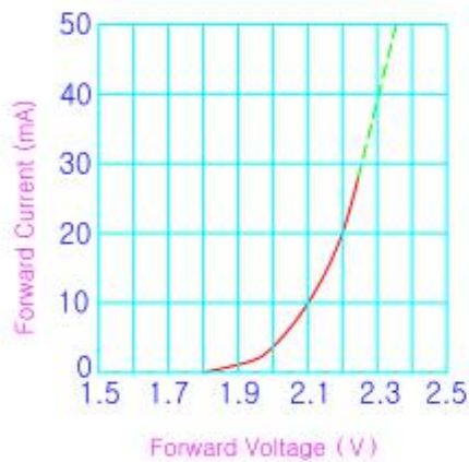
Forward Current Vs. Forward Voltage
