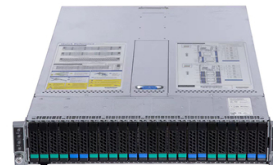
440*770*88mm 2U rack type (12 drawer, 24 drawer chassis optional)
