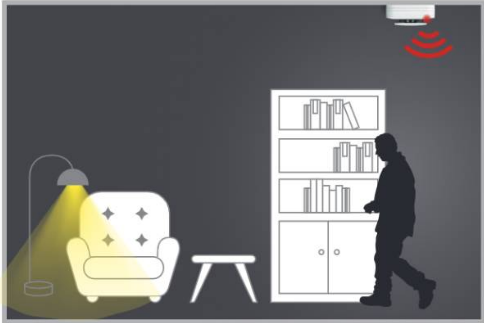
PIR motion sensor for home automation lighting control
