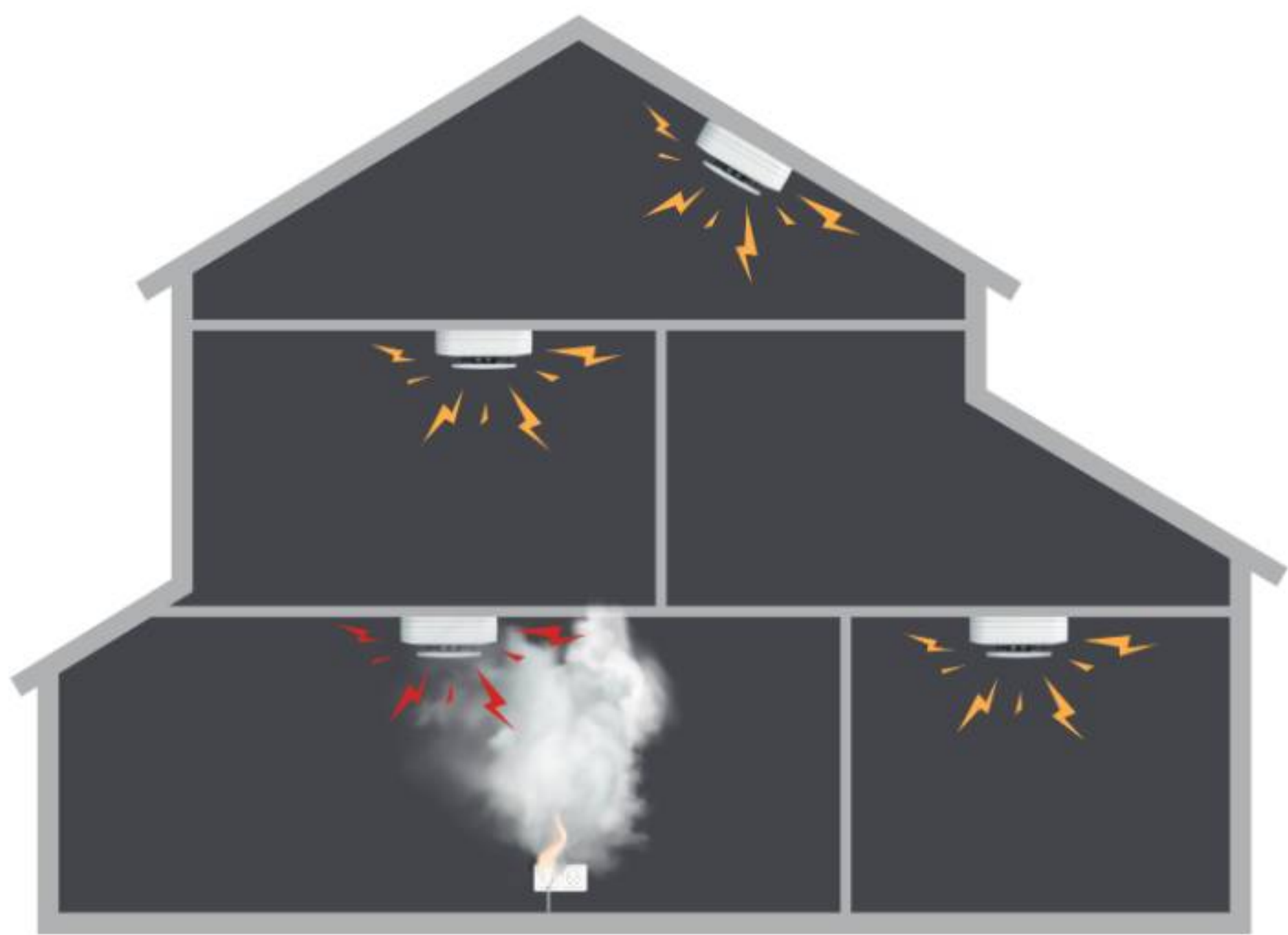
Serial connection enables all connected smoke alarms to sound together when one of them is triggered
