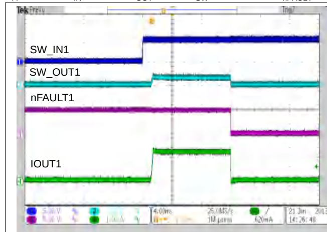
Figure 52. Power Switch1 Enable into Short Circuit
