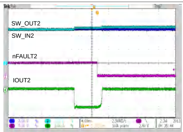
Figure 57. Power Switch2 Reverse Voltage Protection Response
