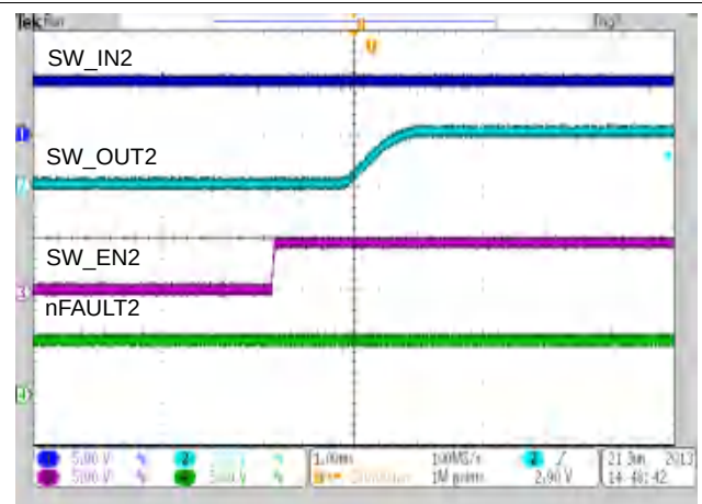
Figure 49. Power Switch2 Turn on Delay and Rise Time
