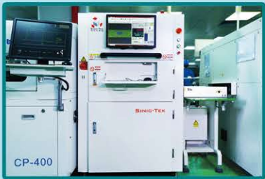
▲ 锡膏检测仪 SPI machine
