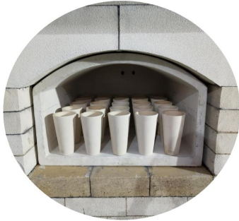
Independent furnace chamber, easy to replace
