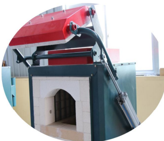
Cylinder controls the oblique opening of the door, more safer.
