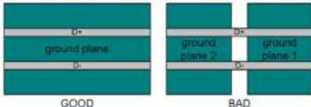
Fig.3-3 RK3126C USB OTG/Host2.0 ground plane guide.
