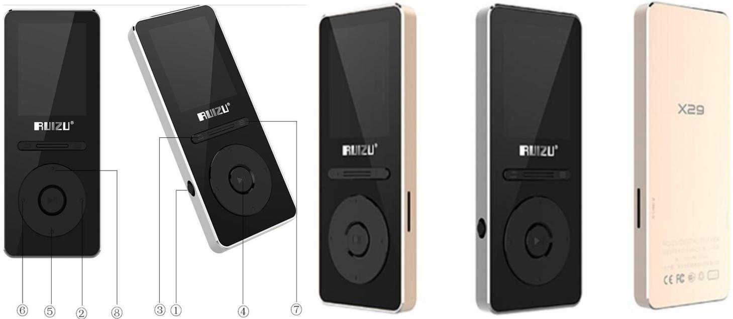
① Power Button : Push the button to " ON " position turn on the player, push the button to "OFF" position turn off the player. When the power button on the "ON"position long press the "Play button" can turn on/off the player
