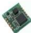
Detecting At Seismic Intensity Level 5 Or Higher Earthquake Sensor D7S
