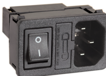
K241335 Panel mount AC socket W/O fuse terminal 4.8mm SW terminal 6.35mm
