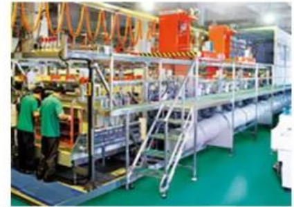
Copper sink line
