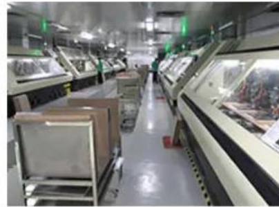
CNC Drilling Machine line
