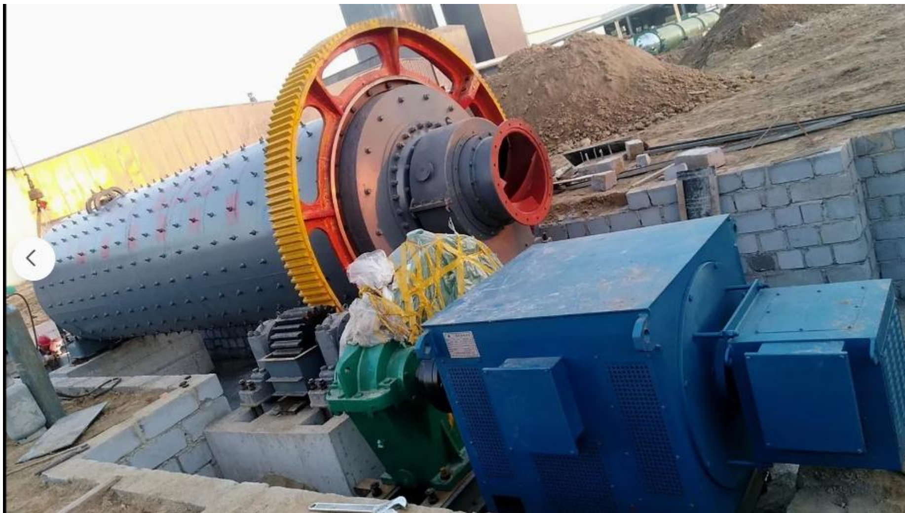
Wet ball mill specifications
