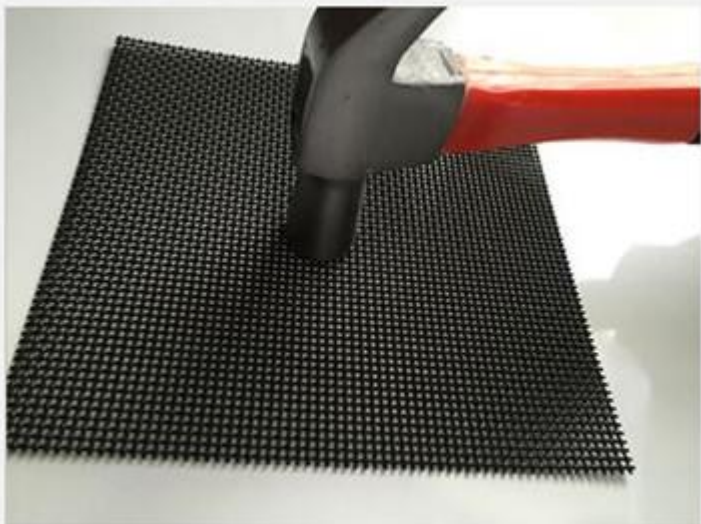
Use a hammer to test the hardness of stainless steel security screen.
