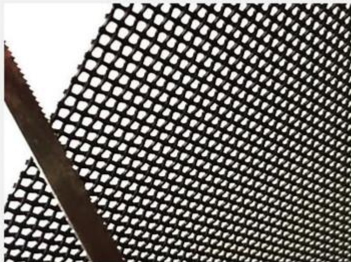
stainless steel security screen can be no deformation through saw test.
