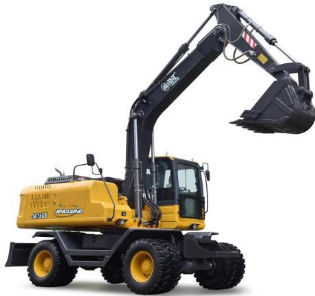
When it comes to JG150S wheel excavator, we bring in three core components from South Korea, rotary motor, multi-tandem valve and two-speed walking motor, providing a strong guarantee of high smoothness and stability.
